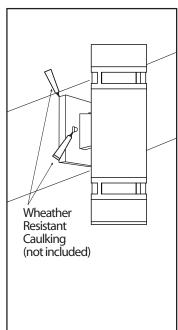
After Installation, seal around the top and side perimeter between the fixture and the wall surface with weather resistant caulking. The bottom should be left un-caulked to prevent moisture build-up. Apply a small amount of weather resistant caulking around the side perimeter between the cap nut and mounting plate.
