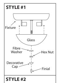
**Fixture** Glass **Fibre** Washer Hex Nut ш Button -STYLE#3 **Fixture**
