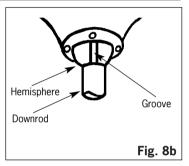
**NOTE:** When installing fan on sloped ceiling, make sure tab on hanger bracket faces towards the top of the slope. Depending on the slope, a longer downrod may be required to prevent fan blades from hitting the ceiling.
